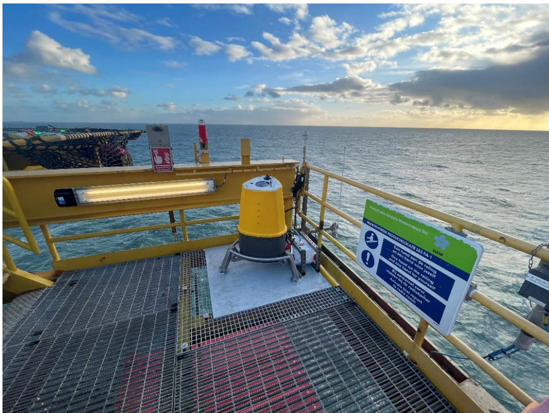
Figure 4.1: ZX300M lidar mounted on top of the accommodation building at L2-FA-1.
