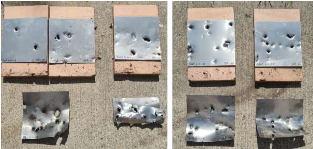
Figure 10 Test 3-3, front target plates are shown at the bottom of the image, back plates with wood backing at the top. Half energetic fragments target plates (left) and inert aluminium fragments (right) and the distance from charge to back plate is 100, 75, 100 and 75 cm from left to right.
