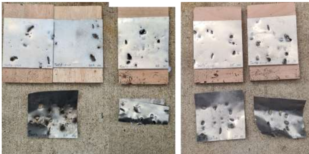
Figure 11 Test 3-4, front target plates are shown at the bottom of the image, back plates with wood backing at the top. Half energetic fragments target plates (left) and inert aluminium fragments (right) and the distance from charge to back plate is 100, 75, 100 and 75 cm from left to right..
