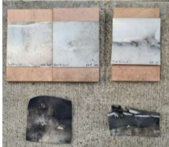
Figure 8 Test number 3-2, with front target plates shown at the bottom, and back plates with wood backing at the top (100 cm distance left and 75 cm right). Target plates were facing the energetic fragments.
