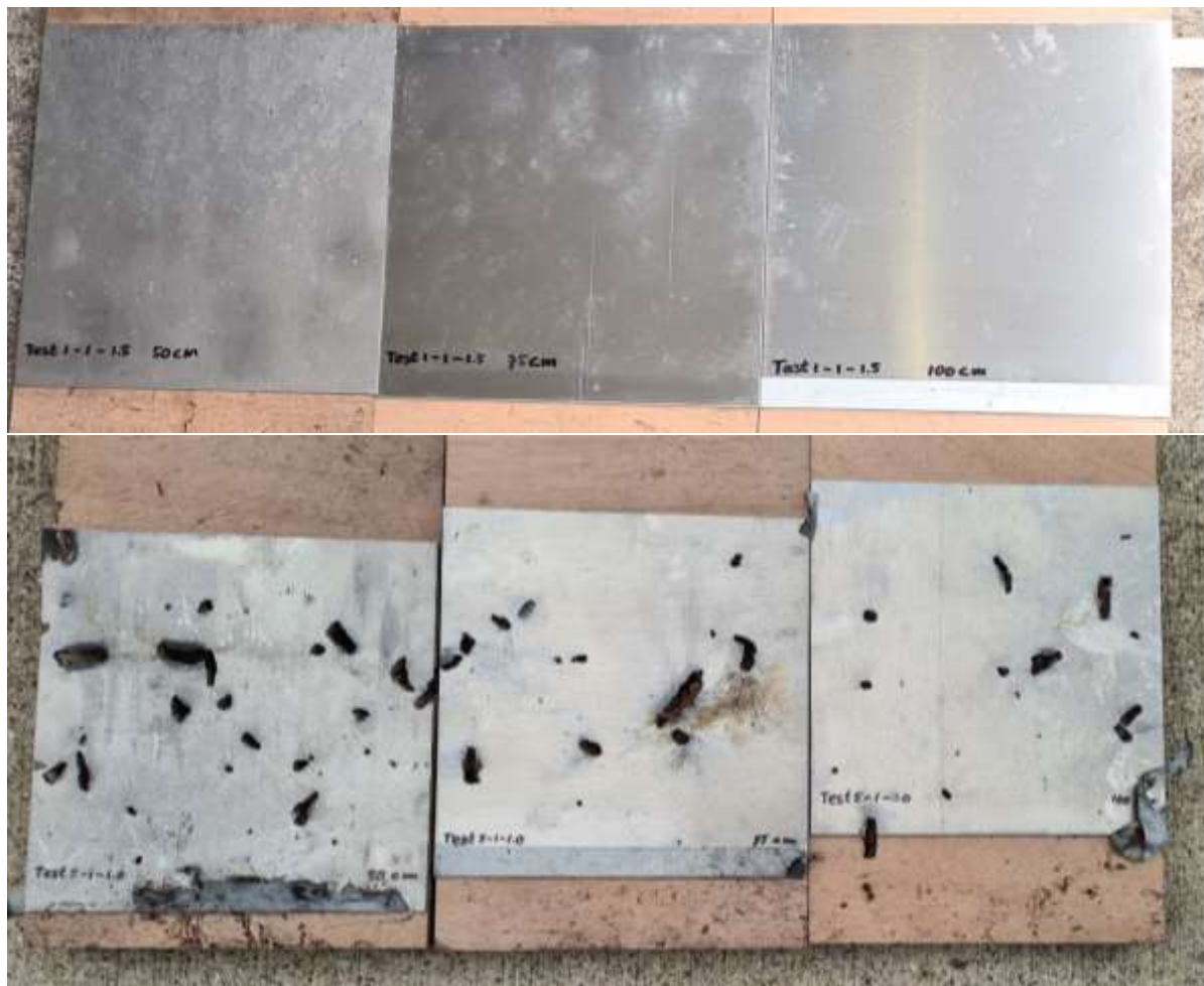
Figure 4 Target plates at 50, 75, and 100 cm in test number 1-1 with plastic charge housing (top), and test number 1-2 with steel charge housing (bottom).
