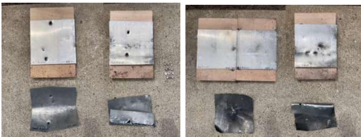
Figure 6 Test number 3-1, with front target plates shown at the bottom of each image, and back plates with wood backing at the top. Target plates facing the inert fragments are shown to the left and energetic fragments to the right.
