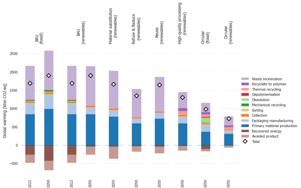
Figure 4.6: Greenhouse gas emissions of the consumer packaging system per scenario, showing the contributions of each processing step. Notes: Thermal recycling sums up pyrolysis and gasification to monomers. “Recyclate to polymer” is an aggregate for the downstream processing steps to create new polymers from the outputs of pyrolysis, gasification, and depolymerisation, namely hydrotreatment, steam cracking and repolymerisation.
