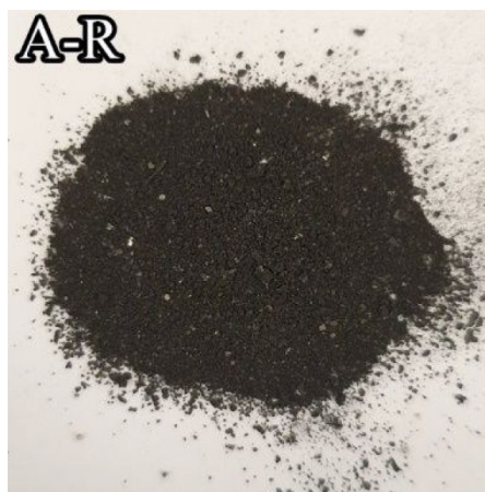
Figure 21: A photo of a black mass sample. The photo is copied from reference (Wu et al., 2020).
