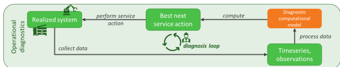
Figure 2.27: The operational diagnosis loop consists of a realized system, observations, a diagnostic computational model and service actions.
