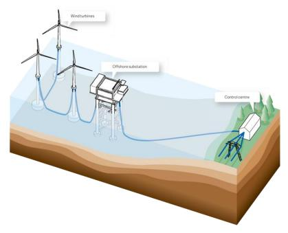
Figure 2.1: Schematic overview of an offshore wind installation.
