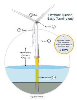
Figure 1: Schematic overview of an offshore wind turbine (Nyserda, 2024)
