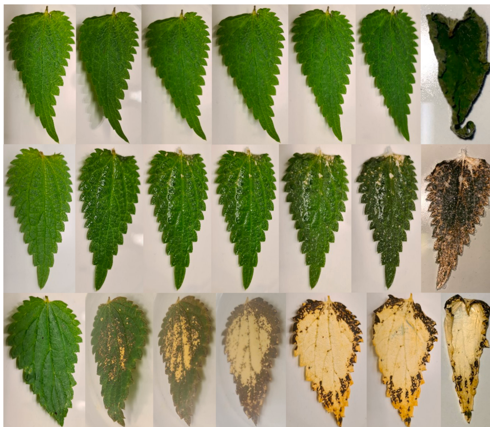
Fig. 2. Blank nettle leaves (top row), leaves immersed in bleach (2nd row) and leaves exposed to 7500 ppm chlorine gas (3rd row). From left to right: after 0 min, 2 min, 5 min, 10 min, 30 min, 60 min, and 24 hours.
