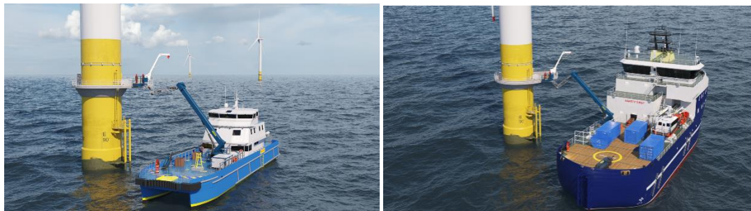
Figure 16. Palfinger OPTS on a CTV (left) and on an SOV (right) (Courtesy of Palfinger)
