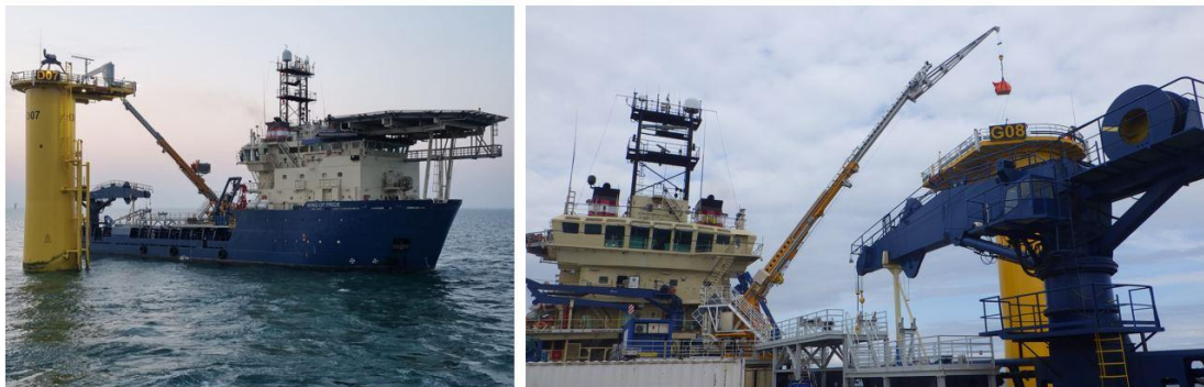
Figure 20. Zbridge W2W with system's elevator (left), Zbridge B2W used as a crane (right) (Courtesy of Z Bridge)
