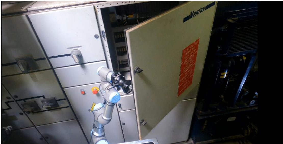
Figure 12. Robot arm remote maintenance in a nacelle - TNO in WCM Zephyros FieldLab
