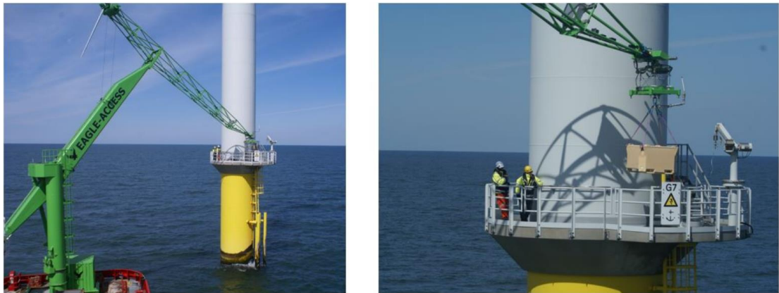
Figure 15. EAGLE ACCESS with an enclosed cabin for technician transfer (left), and used to hoist and deliver cargo (right) (Courtesy of EAGLE-ACCESS)
