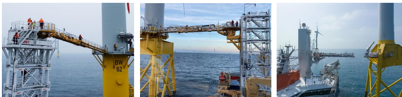
Figure 17. SMST M series (left), L series with Height Adjustment System (middle) (Both courtesy of SMST), and L series together with an Access & Cargo Tower (Photo copyright of Ørsted)
