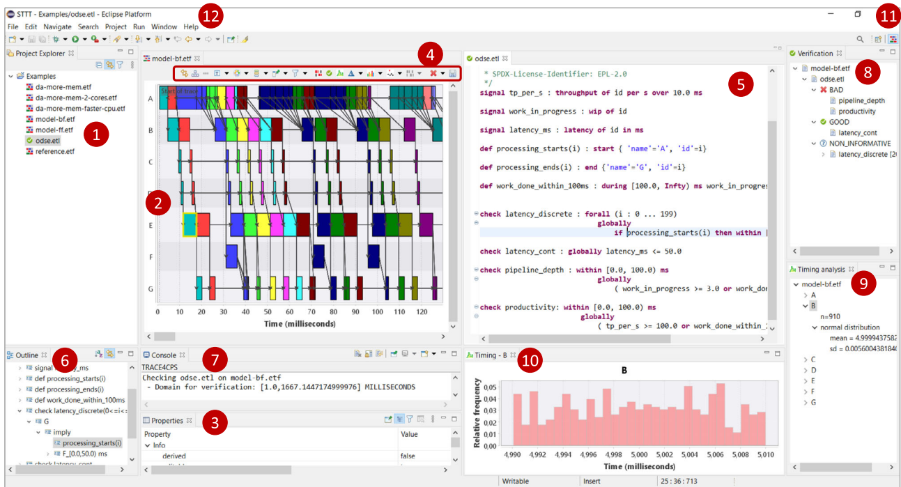
Fig. 3 Overview of the Trace user interface. The file explorer view (1) shows the trace files (Gantt-chart icon) and in this case a single specification file (see Sect. 4) with the green checkmark icon. The Gantt-chart viewer (2) shows trace files. Parts of a trace file – events, dependencies, claims, and signal fragments – can be selected and their properties including the attributes are then shown in the properties view (3). Each Gantt-chart viewer has a toolbar (4) with items to apply techniques, such as the filtering, coloring, and grouping visualization techniques. The various editors support syntax highlighting, etc. In (5), a property specification file is shown. The outline (6) shows the structure of the
