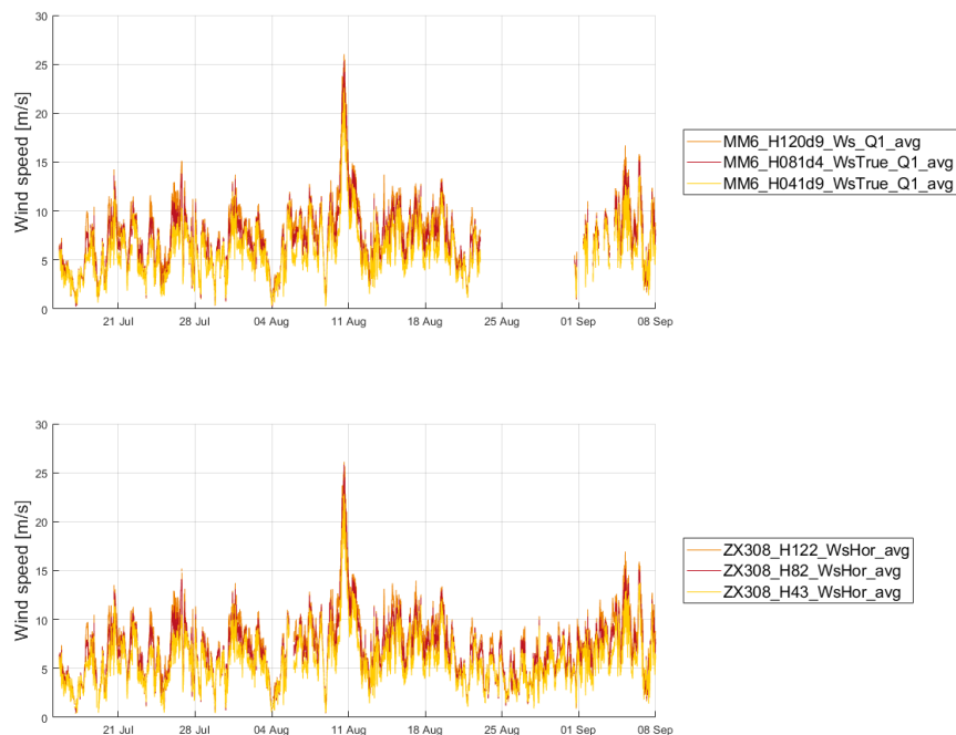
Figure 8: Unfiltered wind speed time series for the comparison heights by the reference meteorological mast at the TNO RSD Verification Facility (top) and the LiDAR (bottom)
