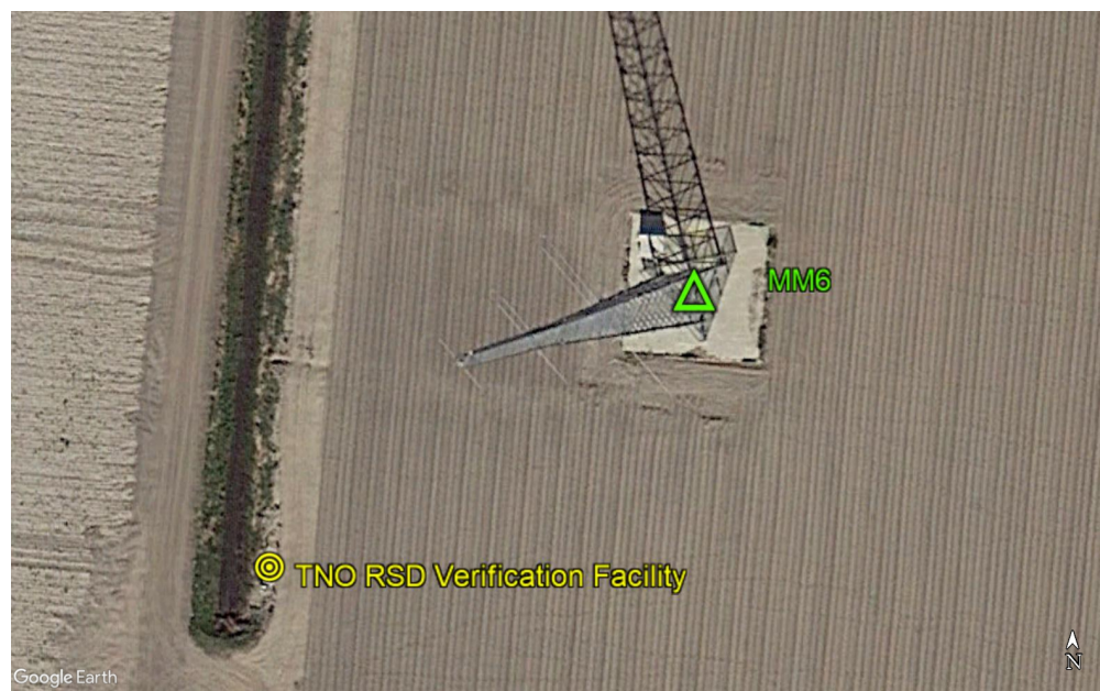
Figure 4: Position of the LiDAR at 49 m from the meteorological mast; indicated in green is the meteorological mast and in yellow the verification platform
