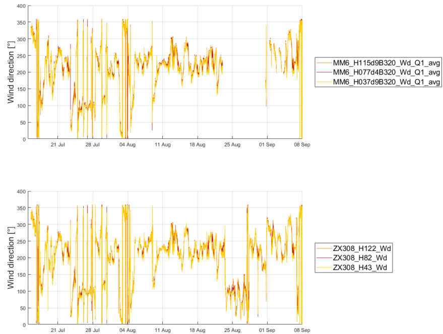
Figure 9: Unfiltered wind direction time series for various heights by the reference meteorological mast at the TNO RSD Verification Facility (top) and the LiDAR (bottom)
