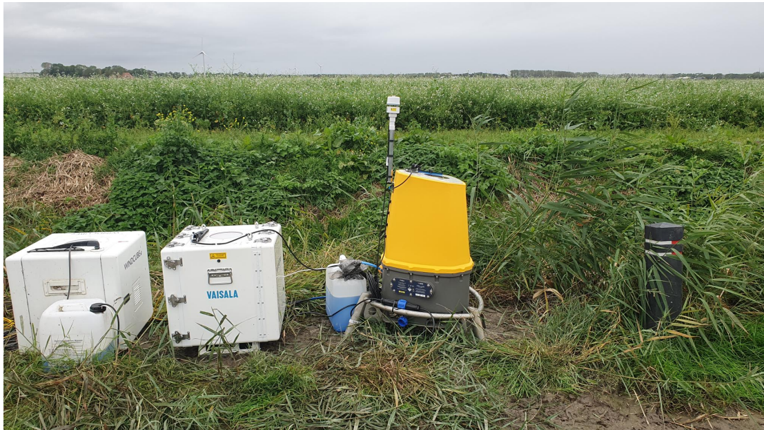
Figure 2.6: ZX 300M ZX563 (right LiDAR in yellow) at the RSD verification location.
