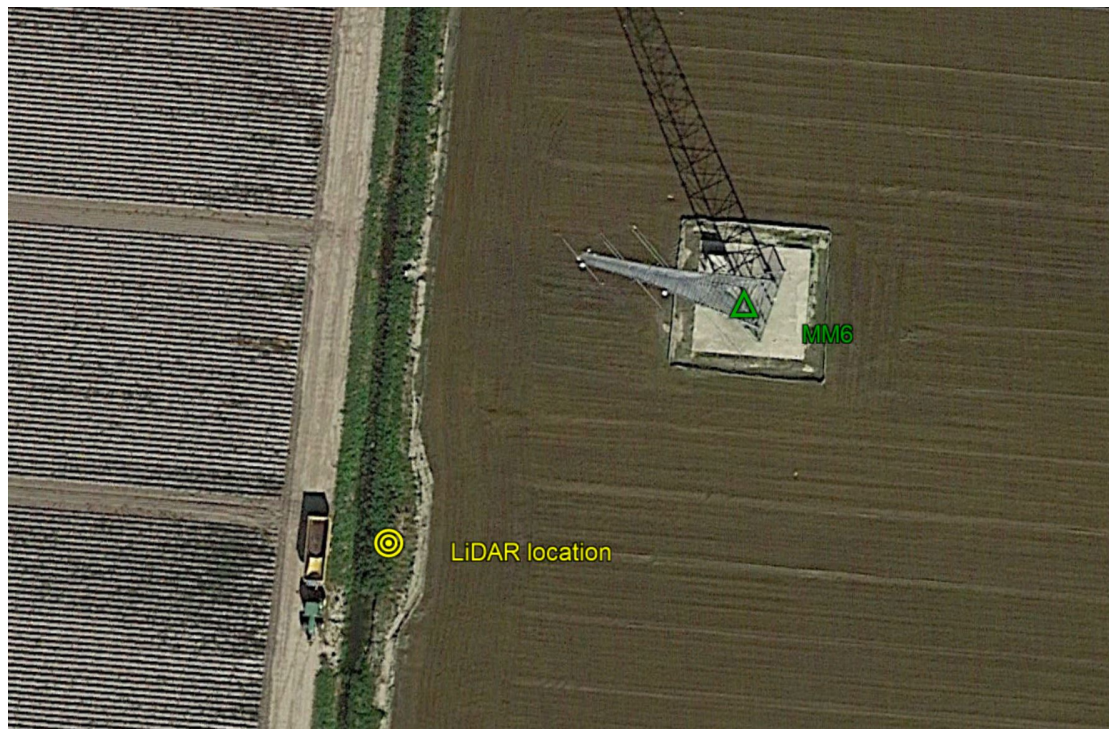
Figure 2.4: Position of the LiDAR at 49 m from the meteorological mast; indicated in green is the meteorological mast and in yellow the verification platform
