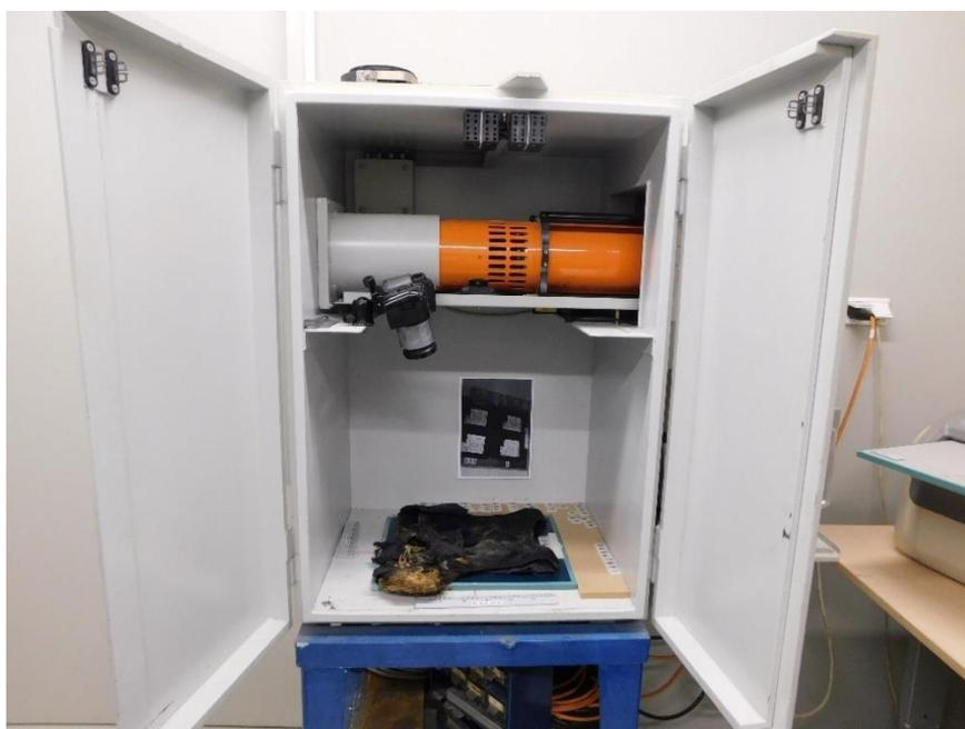
Figure 58 X-ray cabinet. A camera is used for item documentation and identification.
