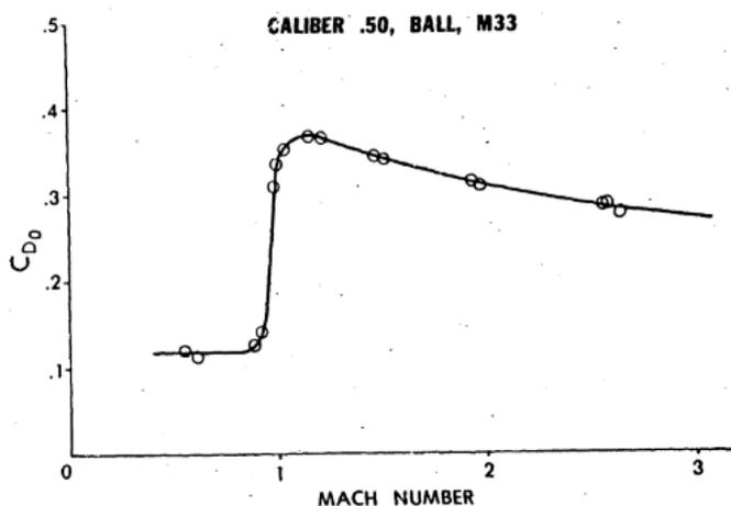
Figure 77 Zero-yaw drag force coefficient versus Mach number, Ball, M33 [McCoy, 1990].
