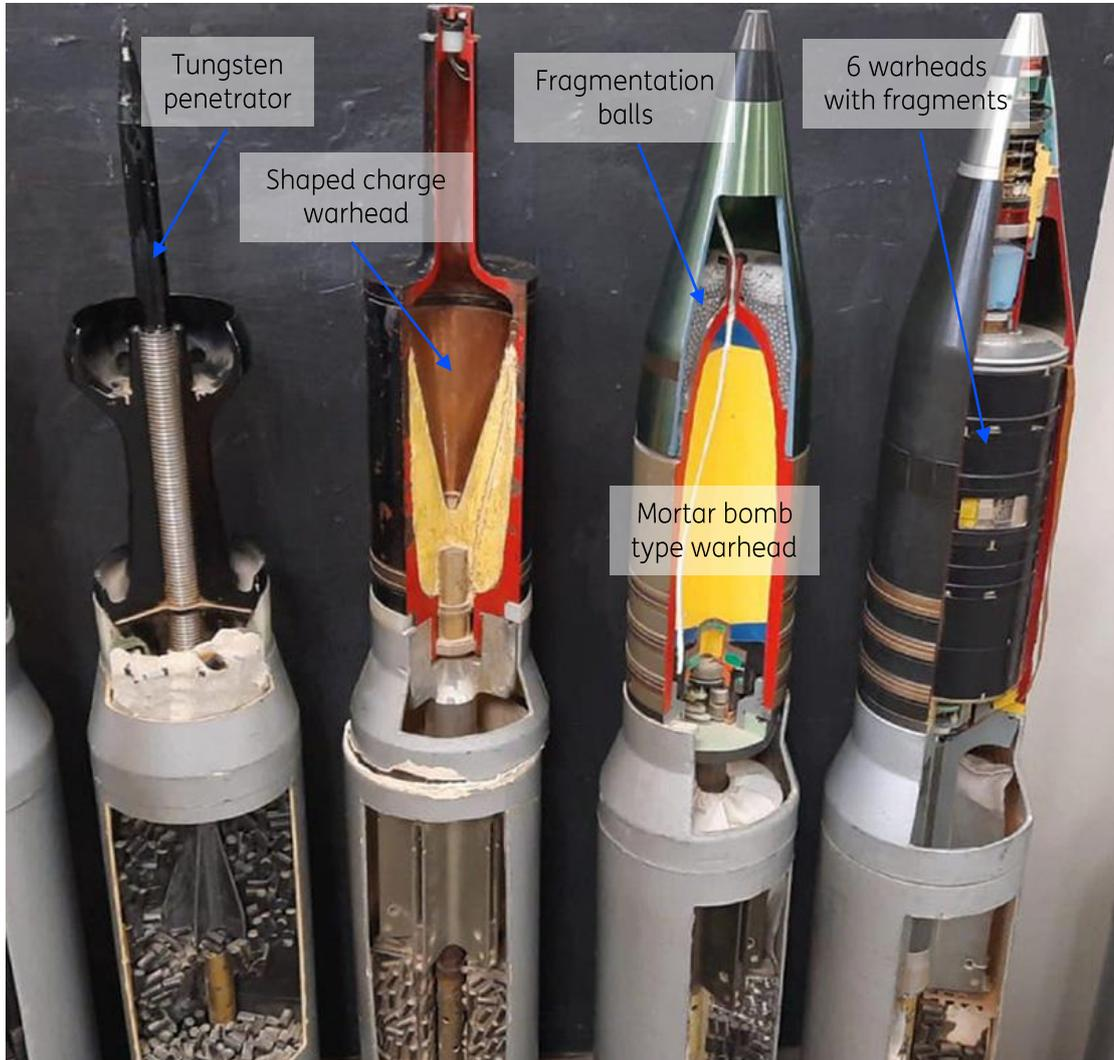
Figure 42 Line-up of Israeli Merkava 120 mm rounds, from left to right: M322 APFSDS-T, M325 HEAT-MP-T, M339 HE-MP-T and M329 APAM-MP-T [X, 2023, 1].
