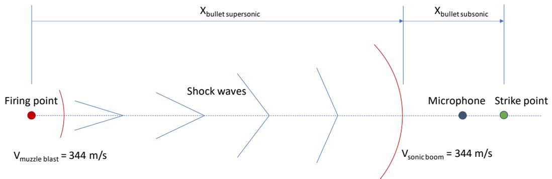
Figure 57 Schematic representation of the TNO model with a supersonic and subsonic region.
