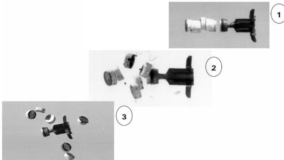
Figure 43 Warhead separation and radial dispersion of M329 APAM in airburst mode [Schirding, 2007].
