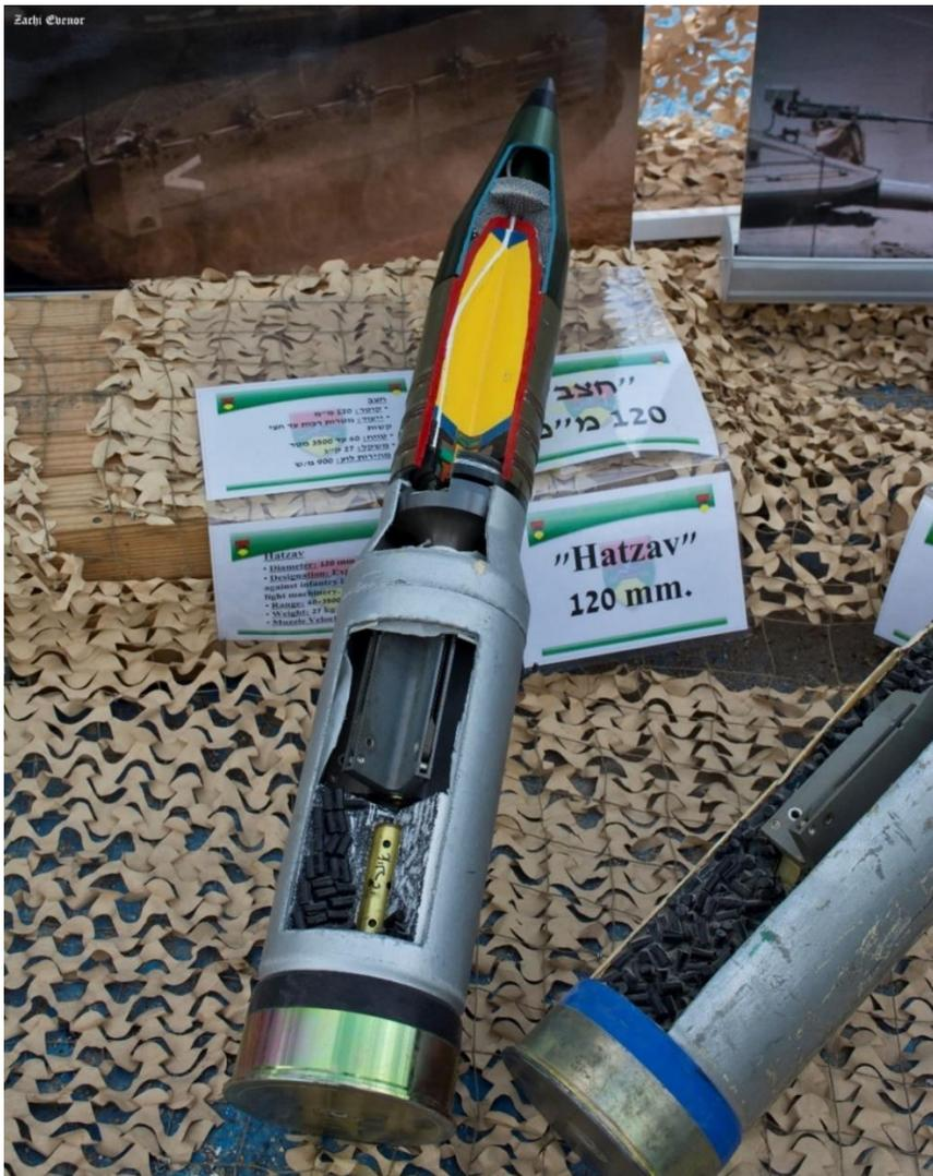
Figure 38 The 120 mm tank round Hatzav [Wikimedia Commons, 2015].
