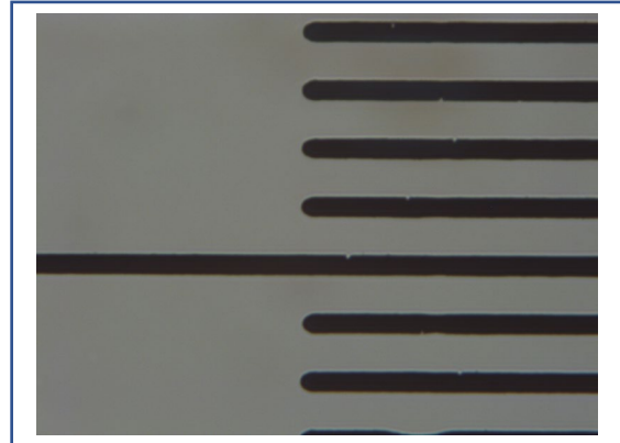
Micrometer scale with 63x objective 1 bar = 10 \mu
