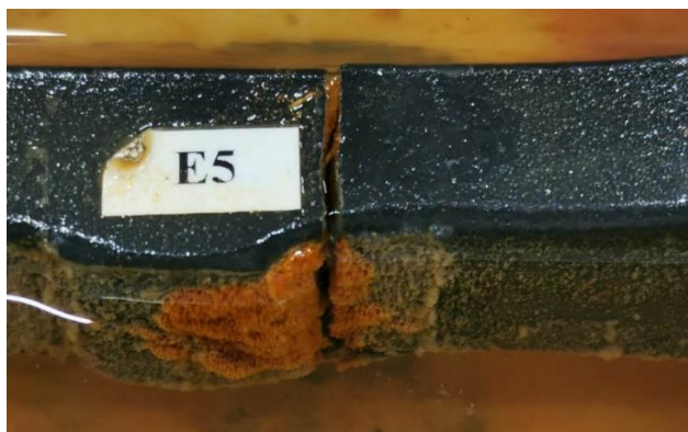
Figure 6.7 – Pre-corroded specimen D-B03 (E5 according Deltares) failed in the corrosion fatigue test.
