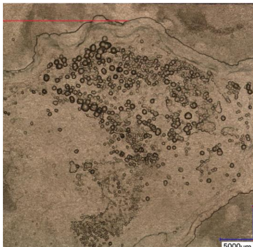
Figure 5.4 – Example of clusters of micro-pits within a large corrosion pit.
