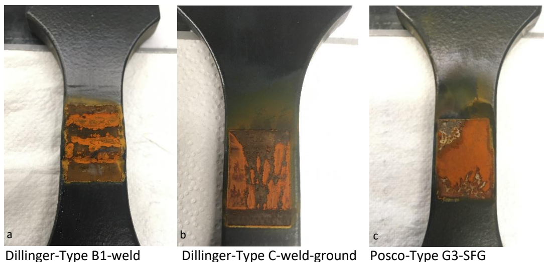
Figure 6.4a to c – Pictures of the pre-corroded areas of the specimens.
