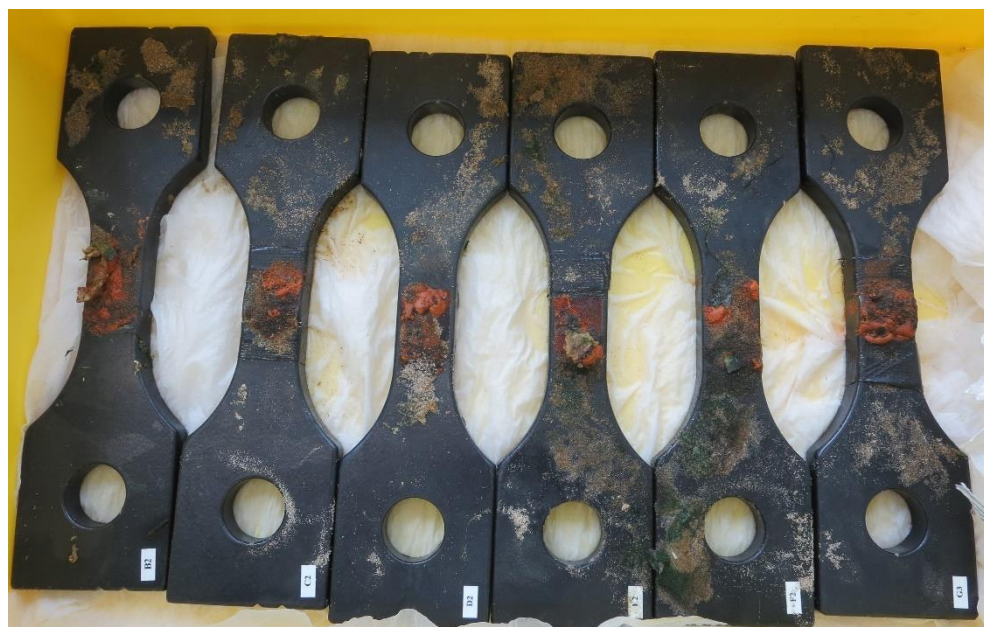
Figure 6.5 – Dogbone specimens pre-corrosion in artificial seawater enriched with micro-biological active bacteria.
