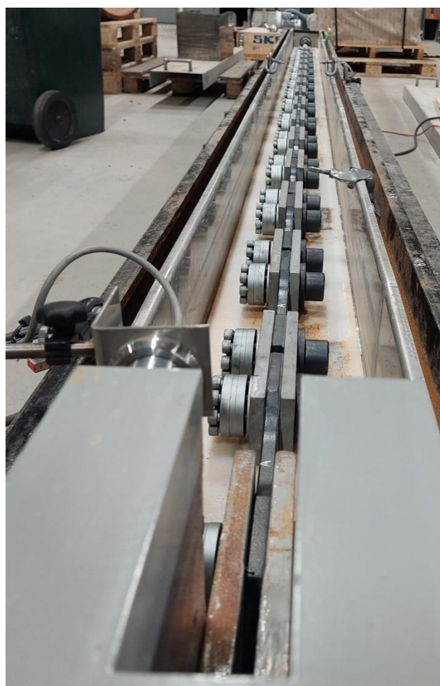
Figure 6.3a/b – The corrosion-fatigue test rig at Vattenfall AB in Sweden.
