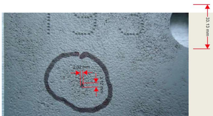
Figure 5.1 – Cluster of microscopic pits on surface, maximum depth of penetration estimated at 0.25 \pm 0.05 mm. The method of assessing the pit dimensions for dataset A is shown (magnification estimated on basis of hole size of 12 mm).
