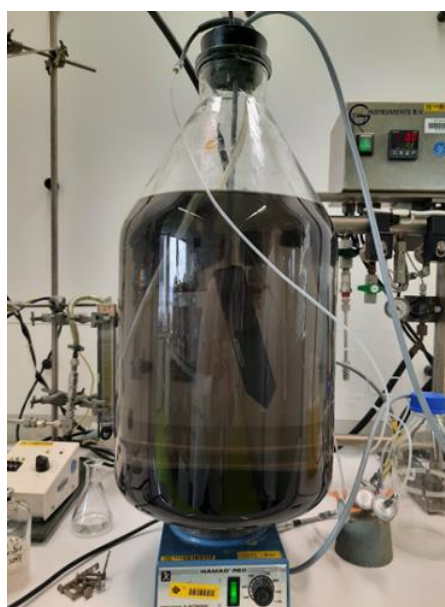
Figure 5.5a/b – a) Flow-through reactor setup with ER probes; b) Stirred vessel incubation with C-rings, ER probes and steel coupons.
