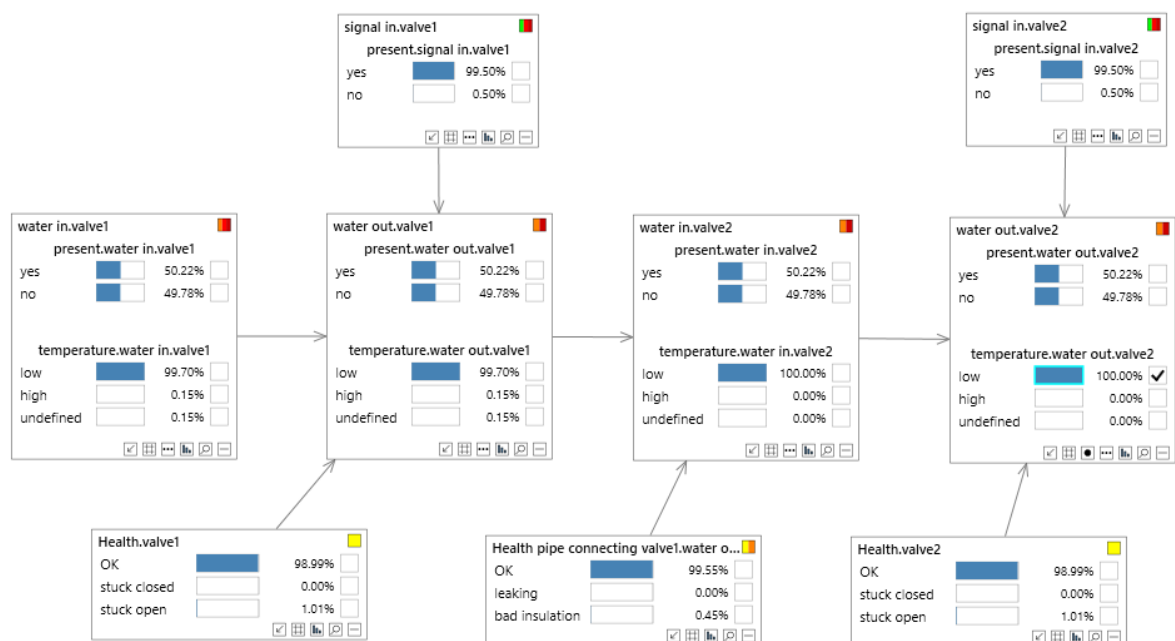
Figure 30 Network without constraints. Even though we measure a low temperature at the output, the network infers that there could be no water.
