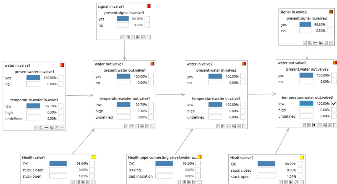
Figure 31 Network with constraints applied correctly infers that low temperature at the output implies water everywhere.
