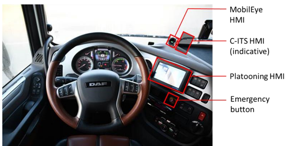
Figure 1-2 Cockpit of the trucks in EcoTwin-3, with the platooning HMI (user interface to (C)ACC functions) and an indicative location of the C-ITS HMI for the current project (Source: D1.2).
