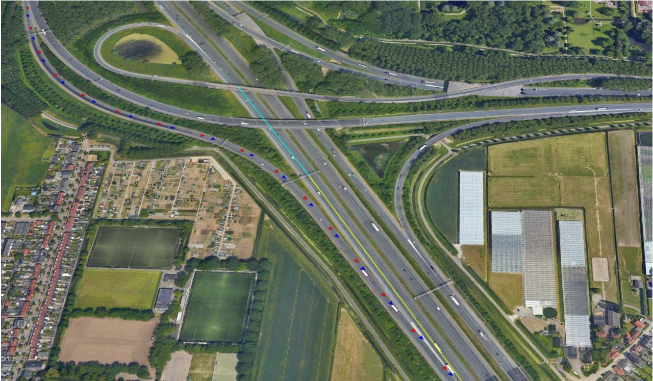
Figure 5-3 Weaving Southbound zone, with the detection zone as a cyan-coloured line, the relevance zone as a yellow-coloured line, and the two trucks visualized with blue and red arrows. On the merging road no detection zone is given.
