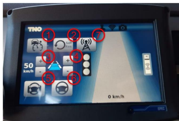
Figure 1-3 The TNO HMI in EcoTwin-3. 1) (C)ACC On/Off; 2) (C)ACC Set/Resume button; 3) Increase/Decrease set speed; 4) Increase/Decrease time gap; 5) Lane Keeping Assist On/Off button; 6) Active Lane Keeping On/Off button; 7) I2V communication On/Off (source: D1.2).
