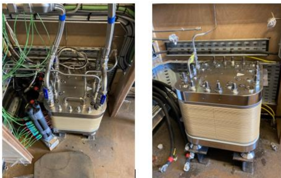
Figure 5: EL500-30 cell commissioning stack in PEM testing system
