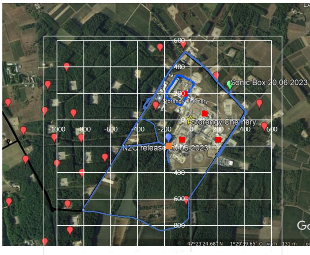
Figure 4-22 Overview of track (in blue) around the site, the sources (in red) and the tracer location (cylinder #11, #15 and #10 in orange) used for the model runs.
