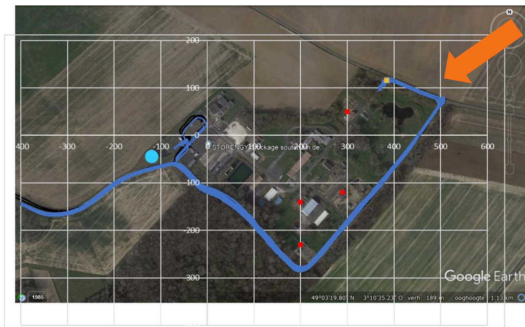
Figure 4-1 Overview of track (in blue) around the site, the sources (in red) and the tracer location (cylinder #17 and #13 in yellow) used for the model runs. The light blue dot represents a manure heap. The orange arrow represent the wind direction.
