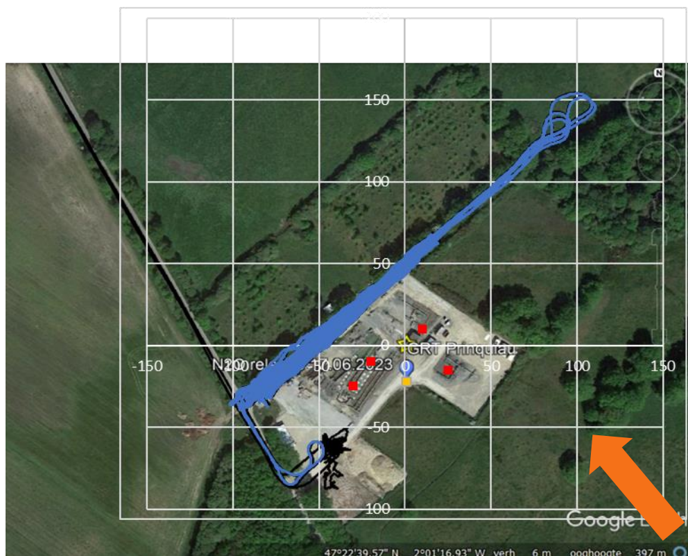
Figure 4-15 Overview of track (in blue) around the site, the sources (in red) and the tracer location (cylinder #15 in yellow) used for the model runs. The orange arrow represent the average wind direction.
