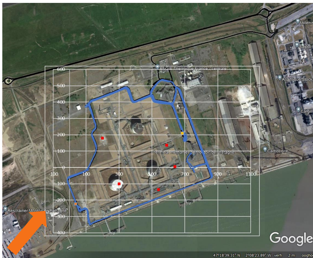
Figure 4-8 Overview of track (in blue) around the site, the sources (in red) and the tracer locations (cylinder #16 in yellow and cylinder #18 in orange) used for the model runs. The orange arrow represent the wind direction, After shifting.
