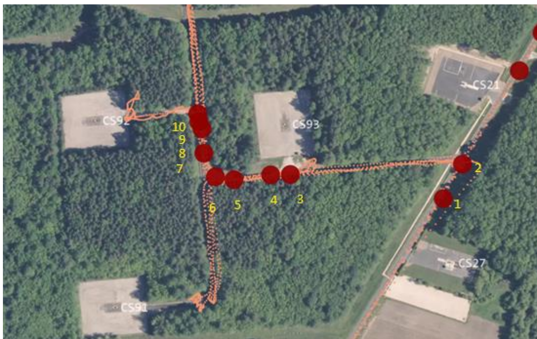
Figure 4-32 Image of the wellheads and where the plumes were observed. The orange small dots indicate the tracks driven by the measurement truck at 2023-06-19 (each dot represent the position of the vehicle for a specific second). The red large dots indicate the locations where a clear plume was observed.
