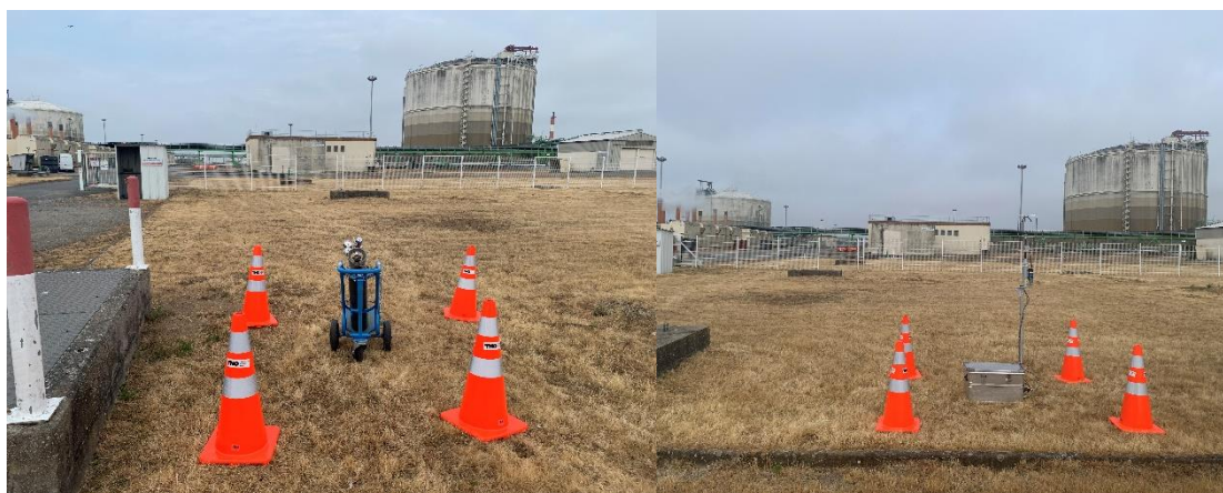
Figure 2-1 Left: set-up N 2 O tracer release; right: 3D sonic anemometer box.
