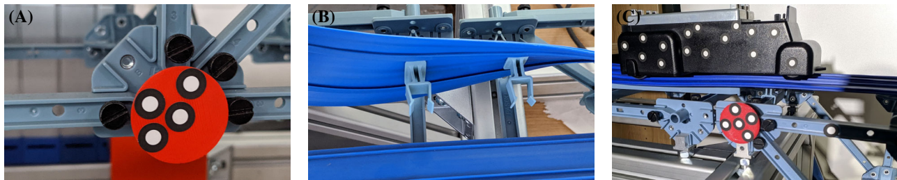
FIGURE 4 PASCO connectors and connection. (A) Beam connection, (B) road connection clip, (C) self driving car for quasi-static loading.
