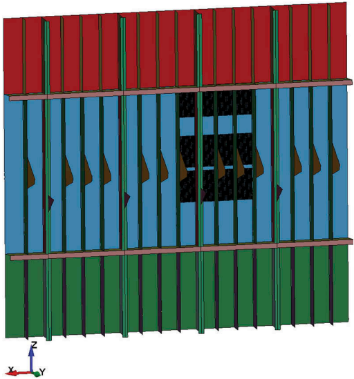
Figure 7. Illustration of impact locations for the stationary patch. Top: IS, middle: UWL, and lower: LWL. Deck has been blanked.
