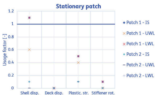
Figure 9. Acceptance criteria results for the stationary load patch analyses.
