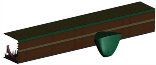
Figure 6. FE model for crash analysis.
