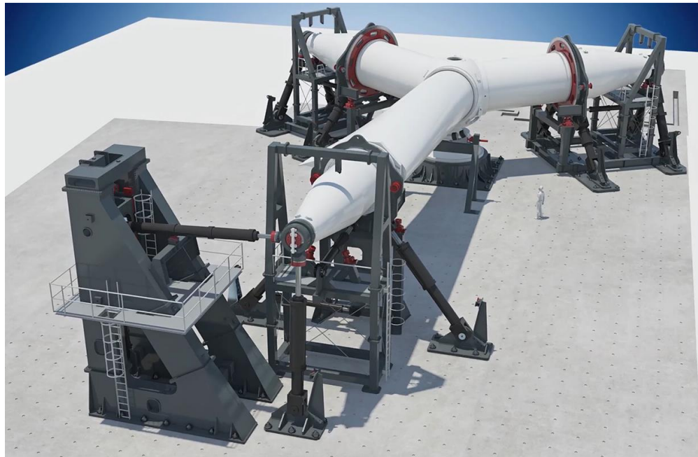
Figure 41 3D illustration of rotor test rig in STRETCH project © LM Wind Power
