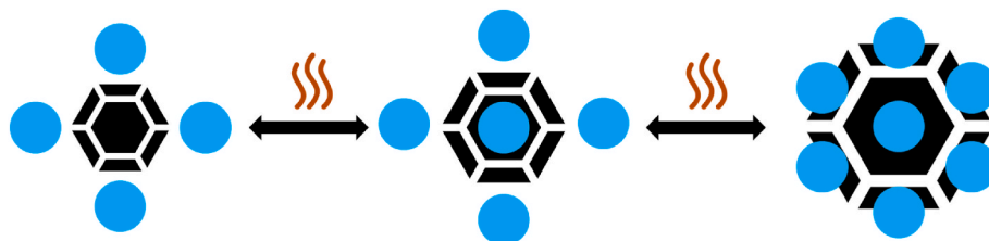
Fig. 1. A principle of hydration-dehydration reaction between salt hydrate (black crystal) and water (blue circle). Q (orange) is the heat released/supplied during the reaction, the image shows two consecutive hydration reactions.
