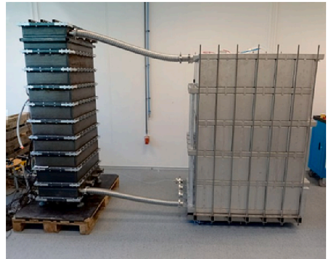
Fig. 2. The prototype of the heat battery [43].
