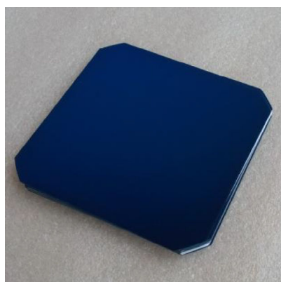
Figure 20. Photograph of the selected solar cell for this work: a 5 in wide SunPower IBC solar cell. On the right, the result from the optical fit based on measurements carried out using the Perkin Elmer Lambda 950 spectrophotometer.
