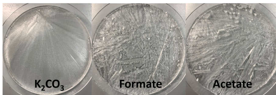
Fig. 10. 2D crystallization test. In the center pure K_2CO_3 ; the others are 5 M % doped K_2CO_3 , with dopants as indicated by label.
