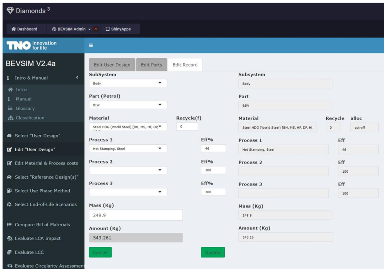
**FIGURE 4** Overview of battery electric vehicle sustainability impact assessment model tool; edit options for a specific sub-system/part by modifying the material, process, mass, recycled content, allocation approach, processing efficiency, and multiple processing steps. In the same screen on the right side, the original design is shown for comparison.
