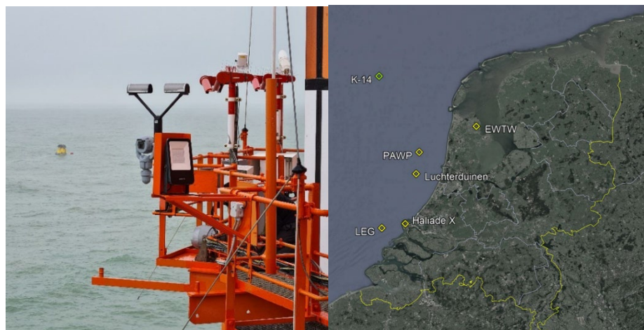
Figure 1.2 Disdrometer instrument installed at LEG platform (left), and the measurement campaign layout (right) for PROWESS project running from 2021 until 2023.
