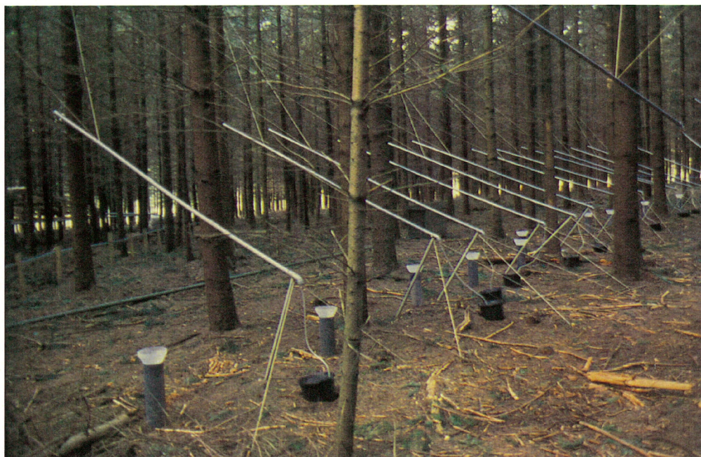
Throughfall sampling at the Speulder forest by means of funnels and gutters.
