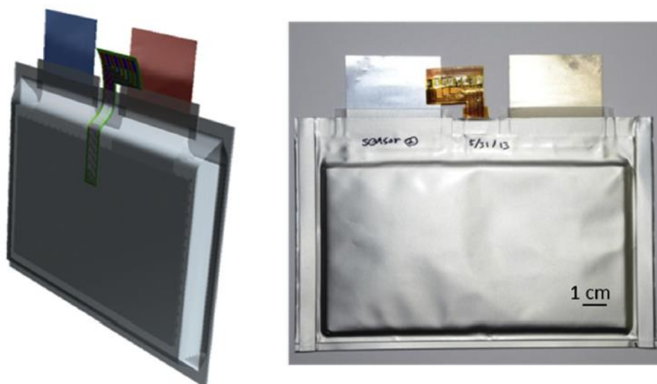
Figure 5: Position of micro temperature sensors in lithium-ion secondary battery.
