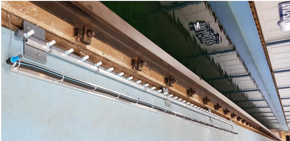
Figure 6.1: Photo of the 'nozzle' and 'porous' hoses, next to MARIN's Concept Basin.
