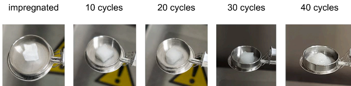
Fig. 19. Visual inspection of the LiCl-polymer composite before and after cycling. Note that the first picture has salt in the anhydrous form whereas the other pictures contain the salt in deliquescent form.
