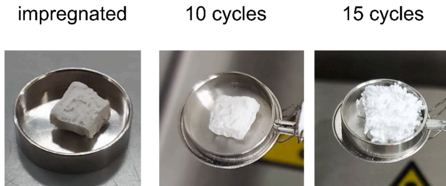
Fig. 16. Visual inspection of the CaCl 2 -polymer composite before and after cycling. Note that the first picture has salt in the anhydrous form, whereas the other pictures contain the salt in hydrous form.
