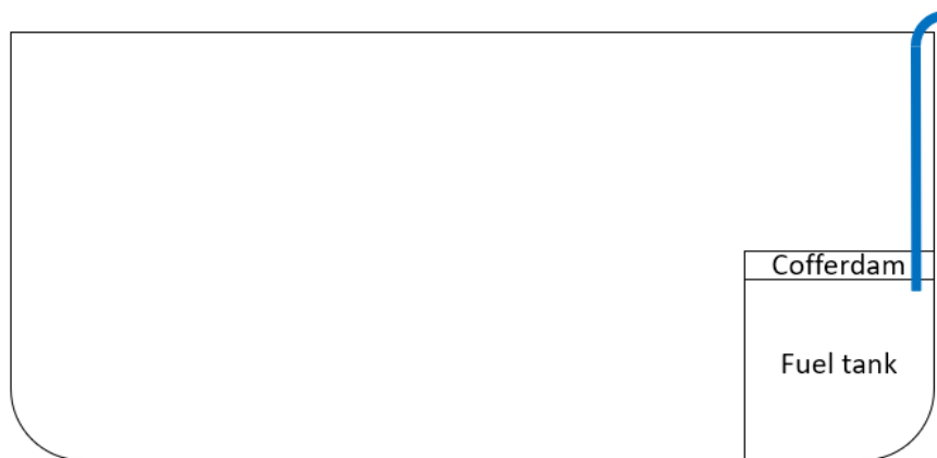
Figure 4.10: Cross-section with schematic illustration of methanol venting over the side of the ship
