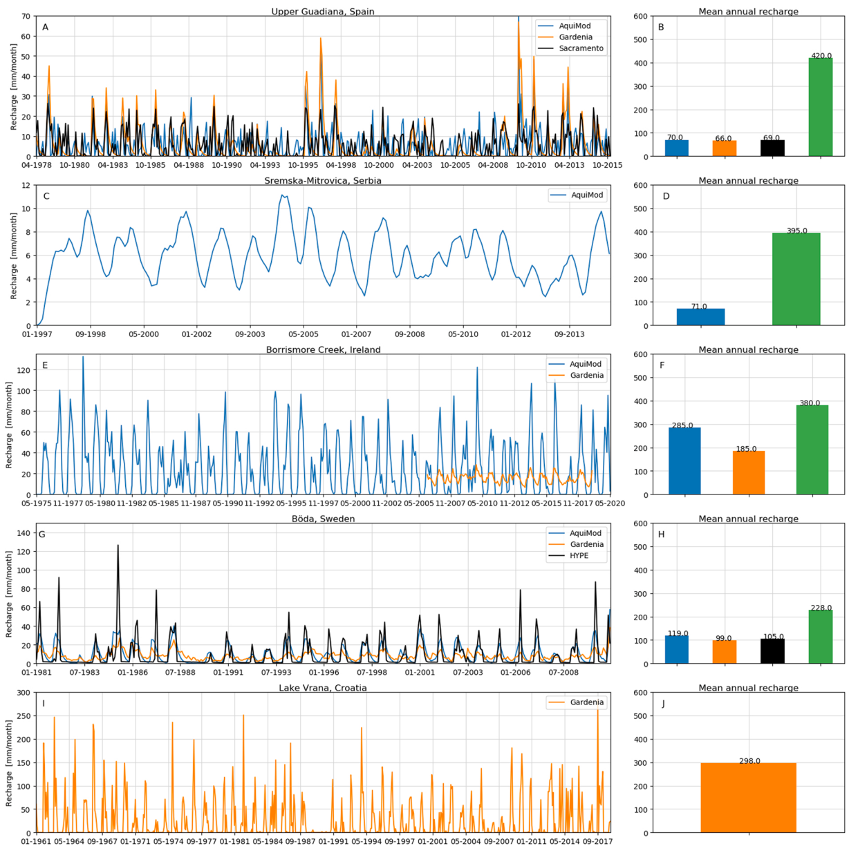
Fig. 5. Simulated recharge values (mm/month) with GARDÉNIA, AquiferMod and any local model present in the case study (left), with mean annual recharge values for the same simulations (right) with the addition of Metran (green bar) that only provides results on annual basis. Selected results are shown for the four selected case studies: Spain (A), Serbia (C), Ireland (E), and Sweden (G).
