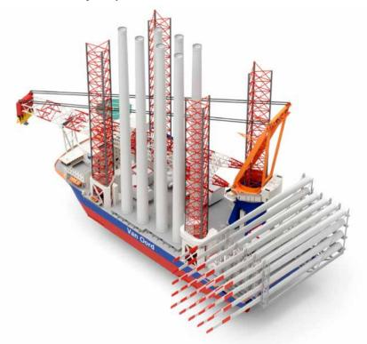
Figure 4: Jack-up vessel powered by methanol and ordered by Van Oord.
