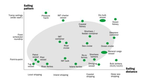
Figure 13: Ship types thought to be suitable for methanol propulsion
