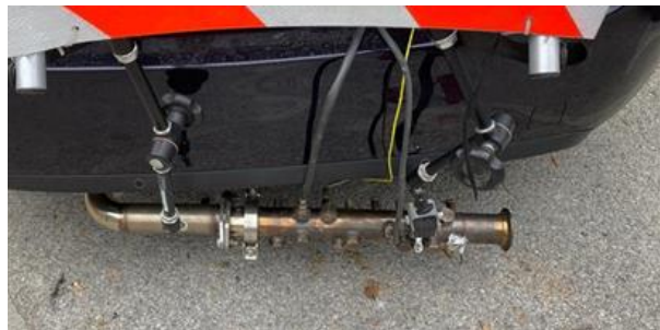
Figure 3.4: SEMS installation on the LD1, the exhaust sensors were placed in an extension pipe supported on the back of the vehicle.
