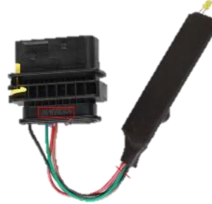
Figure 4.12: Type 2 SCR emulator tested by Bosch
