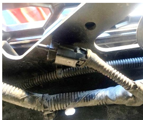
Figure 4.7: Truck AAT sensor located behind the grill
