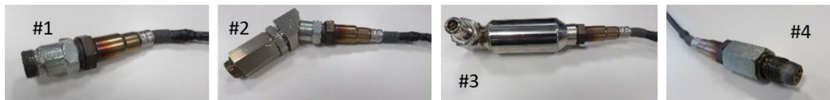
Figure 4.1: TWC lambda sensor spacers: #1 simple spacer, #2 spacer with metallic catalyst, #3 spacer with Euro 4 catalyst, #4 spacer with ceramic catalyst
