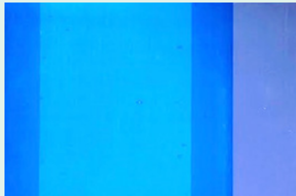
Figure 13. Ruthenium deposited on an aluminium oxide coated wafer.
