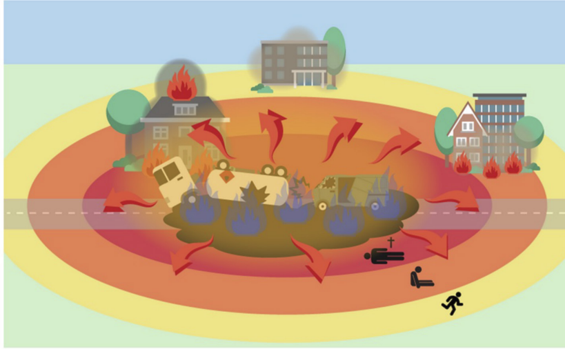
Figure 32: Schematic representation of pool fire, taken from [ https://www.scenarioboek.nl/ ].
