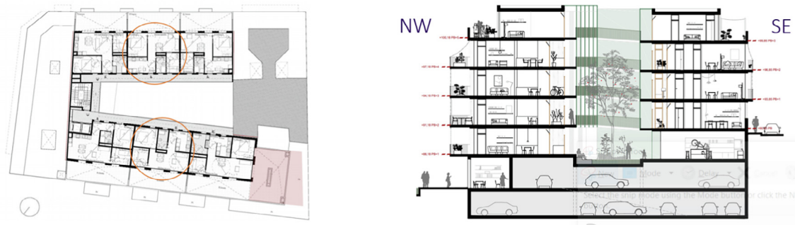
Fig. 4. Architectural drawings of the floor plan of the Barcelona demo site building's attic floor (left) and the elevation section (right). Apartments that were modelled in detail are circled with orange. (For interpretation of the references to colour in this figure legend, the reader is referred to the web version of this article.)
