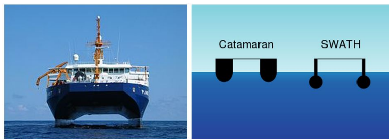
Figure 7: A SWATH vessel (left) and the distinguishing narrow waterline hull design (right)
