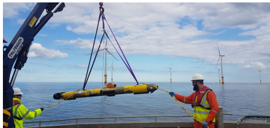
Figure 14: A consortium comprising of the R&D UK Centre of EDF Energy, UTEC, an Acteon company, and Partrac Ltd completed an offshore trial designed to assess the performance of a commercial UUV (UUV) for mapping seabed bathymetry.
