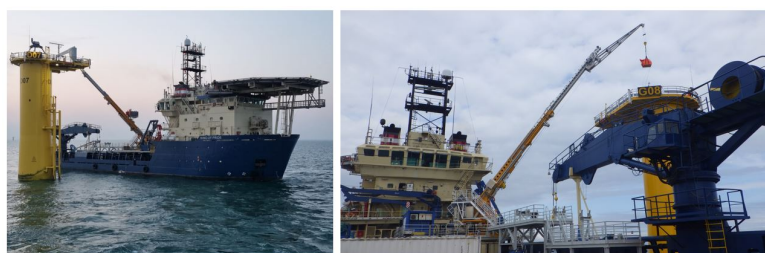
Figure 26: Zbridge W2W with system's elevator (left), Zbridge B2W used as a crane (right)
