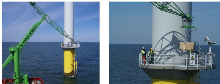
Figure 21: EAGLE ACCESS with an enclosed cabin for technician transfer (left), and used to hoist and deliver cargo (right)
