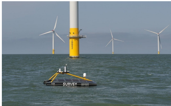
Figure 13: XOCEAN's XO-450 unmanned surface vessel (USV) performing seabed survey.
