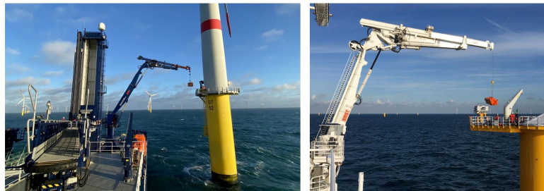
Figure 23: SMST motion compensated crane in operation (Courtesy of SMST)
