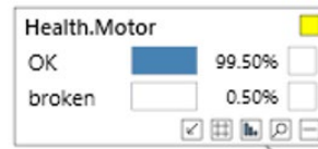
Figure 20 Health node of the Motor component in the Bayes net. Here, the Motor has one generic failure state "broken".
