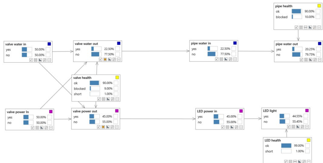
Figure 40 Bayes Net of the electrical valve example without considering upstream behavior
