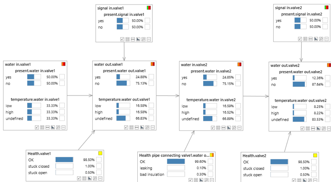
Figure 26 Network with multiple variables per node.
