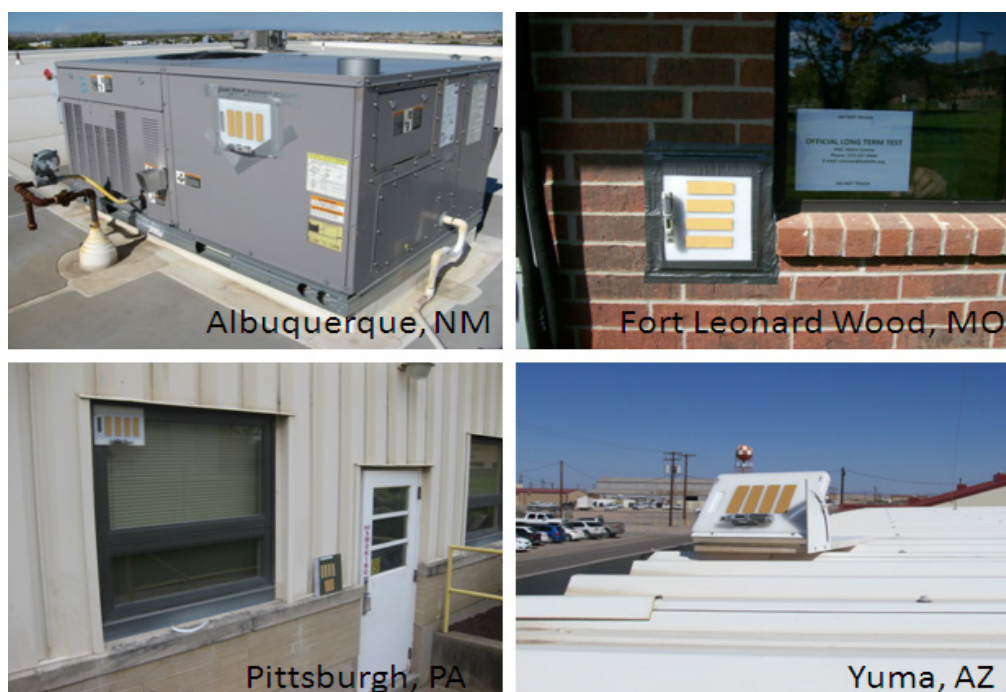
Figure 4-10: Coating Samples Were Exposed in Four Locales for a Period Up to 6 Weeks.
