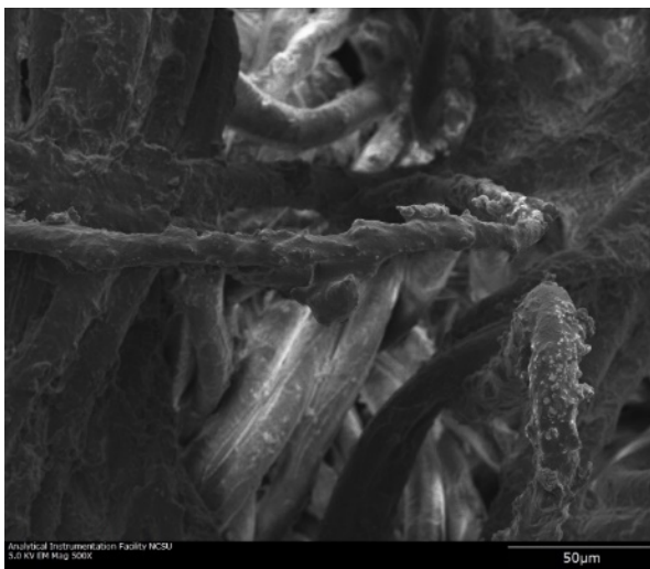
Figure 3-13: \text{NaHCO}_3 Can Increase the Roughness of the Surface Due to the Air Generated During Heating.
