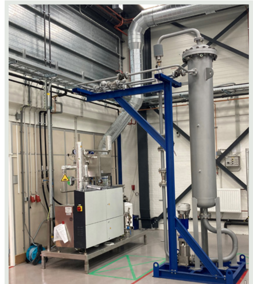
High temperature PCM TES prototype at TNO Laboratory, Petten, Netherlands.
