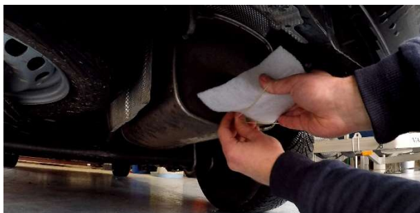
Figure 3-5: Exhaust PM with filter test step 3 (left) and step 7 (right)
