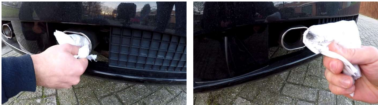
Figure 3-7: Exhaust PM swipe test step 1 (left) and step 4 (right)
