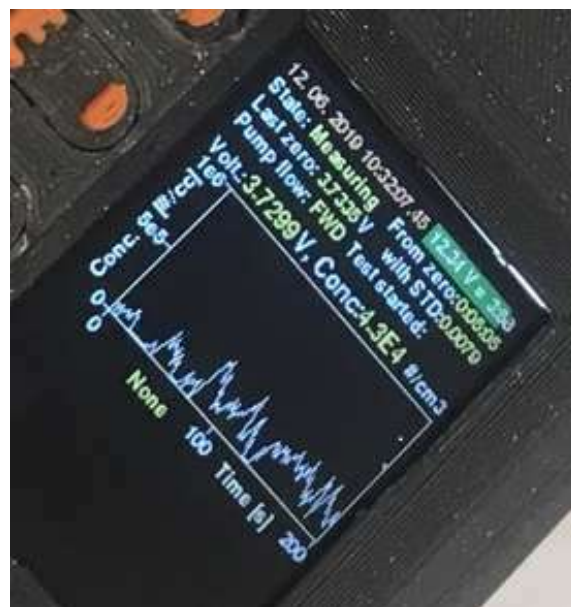
Figure 3-12: DPF inspection tool in action
