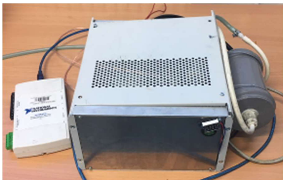
Figure 4-2: Grey wastewater pipe with an ionization smoke detector inside
