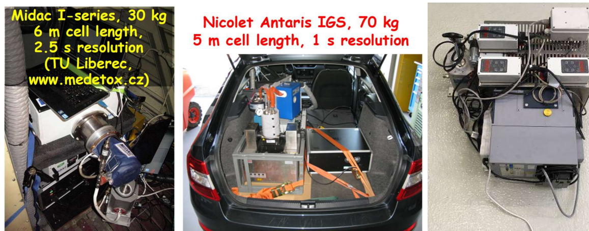
Figure 4-7: FTIR instruments used on-road: MIDAC I-series, (left), Nicolet Antaris IGS (middle) and Bruker Matrix (right)
