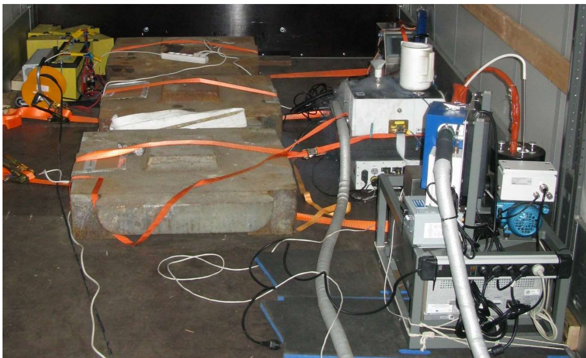
Figure 4-8: FTIR analyzers Nicolet( front) and MIDAC (back) in the cargo space of a 12-ton Euro VI diesel truck during an evaluation test at the Czech Technical University in Prague (3 steel ingots corresponding to approx. 50% payload are in the middle and batteries are in left front)
