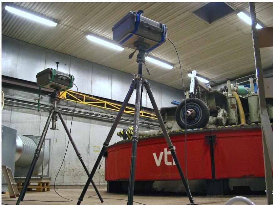
**Figure 7.10. The VTI circular road simulator.**
