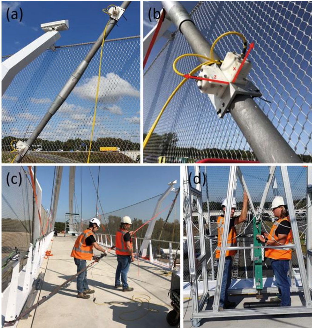
Fig. 2 Pictures of the setup of the measurements: a Two measurement positions along the length of the cable, b at each location two accelerometers were placed, measuring in two directions. c The step-relaxation excitation of the cables was realised with a lashing strap. d The deck was excited with a 250 kg impact hammer
