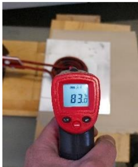
Figure 9. Temperature reading of the induction heating.
