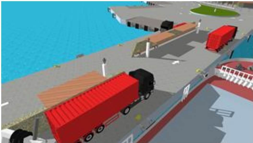
Figure 9. An indication how the situational view could look like. It is a real-time digital twin rendered by IOSS to enable an operator to view an autonomous ship's current situation through virtual reality.
