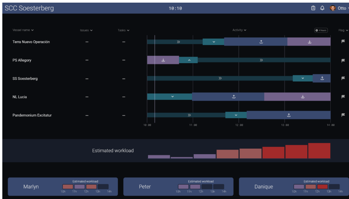
Figure 7. Our concept for the global view of an operator's interface. It lists all ships the operator is currently responsible for and detailed information such as open tasks, ship phases, and the expected workload of him-/herself and direct colleagues.
