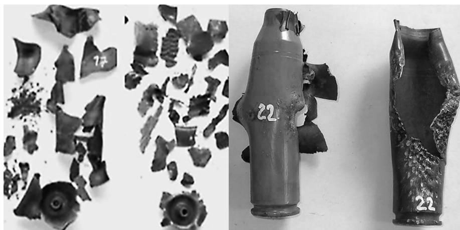
FIG. 18: Shaped charge jet (left cartridge remains) and hot fragment responses (right cartridge remains) in the German LSP test. Left picture: typical response of conventional propellants with NG. Right picture: response of next-generation SCDB (surface-coated double-base) propellant (reprinted from Andres et al. with permission from Nitrochemie, copyright 2006).
